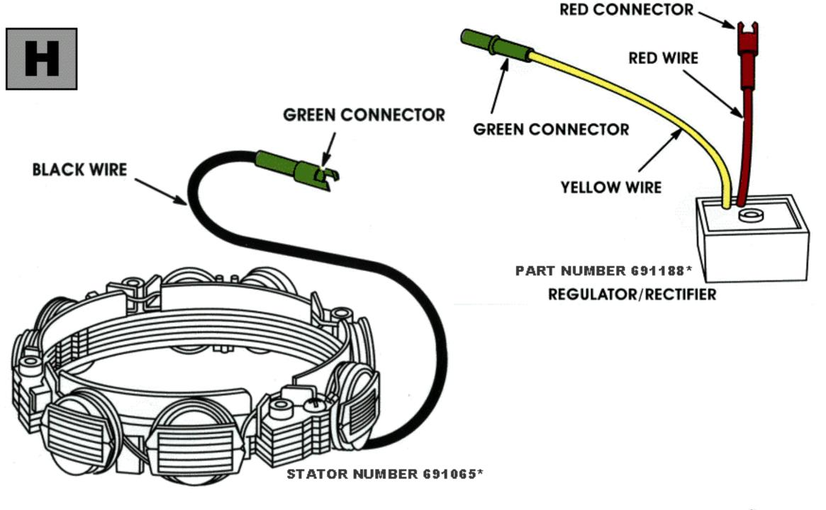
@3600 RPMs-9A Alternator 40 Volts AC(Min) at Stator; 9A, DC Regulated-red wire
