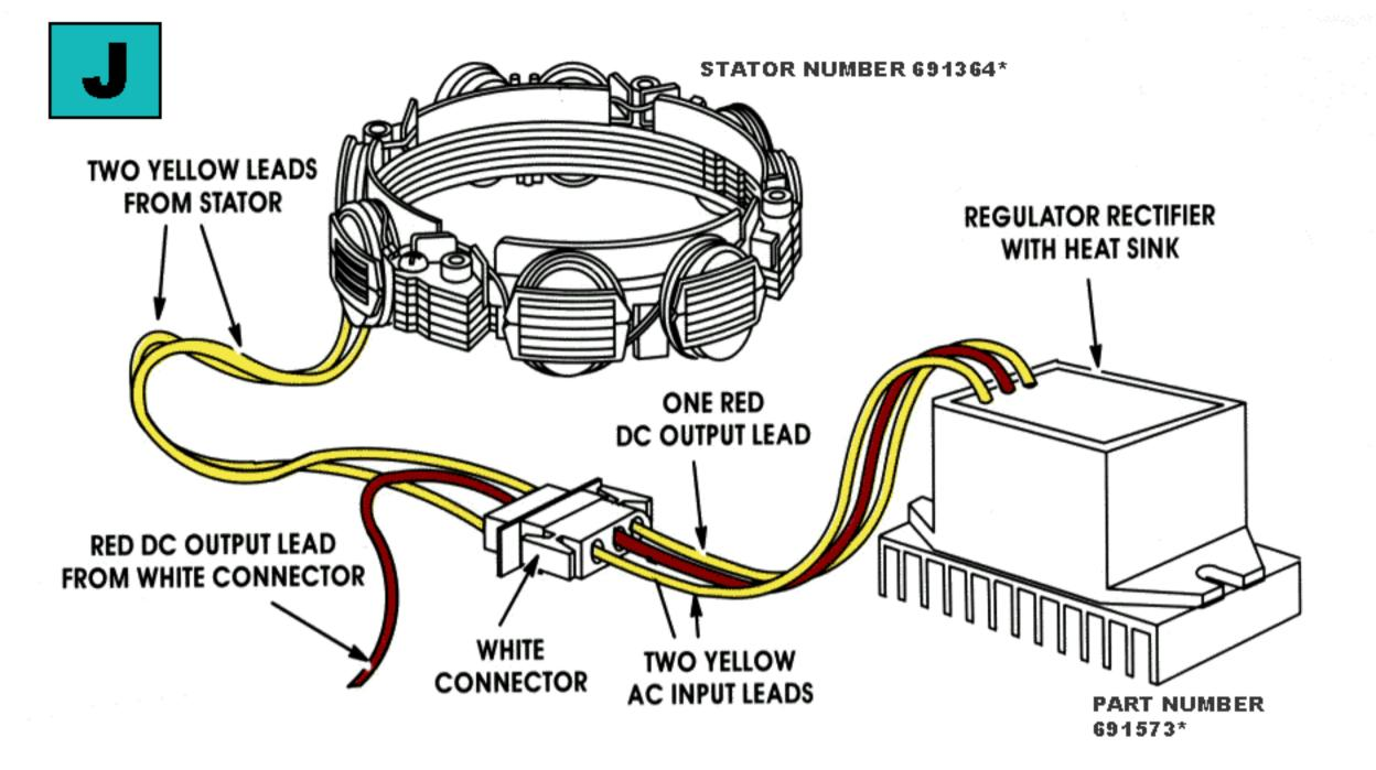
@3600 RPMs-20A Alternator 29 Volts AC(Min) at Stator; 20A, DC Regulatedred wire
