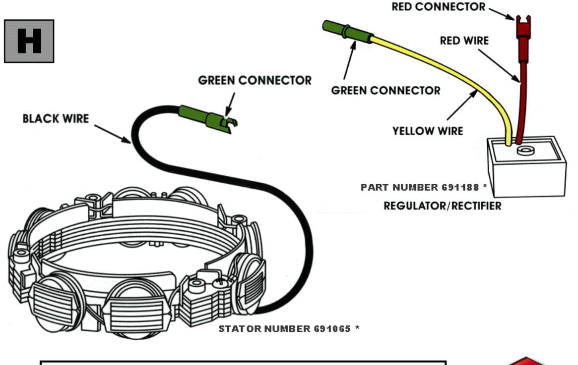
@ 3600 RPMs-5A Alternator 28 Volts AC(Min) at Stator; 5A, DC Regulated-red wire
