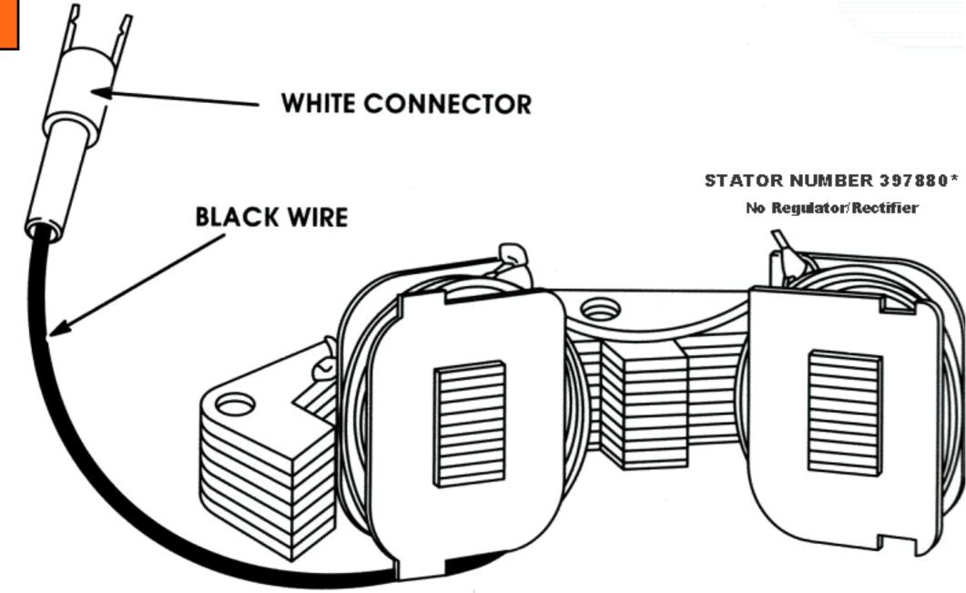
System 3/System 4 .5A, DC Unregulated (Output at 2800 RPM)
