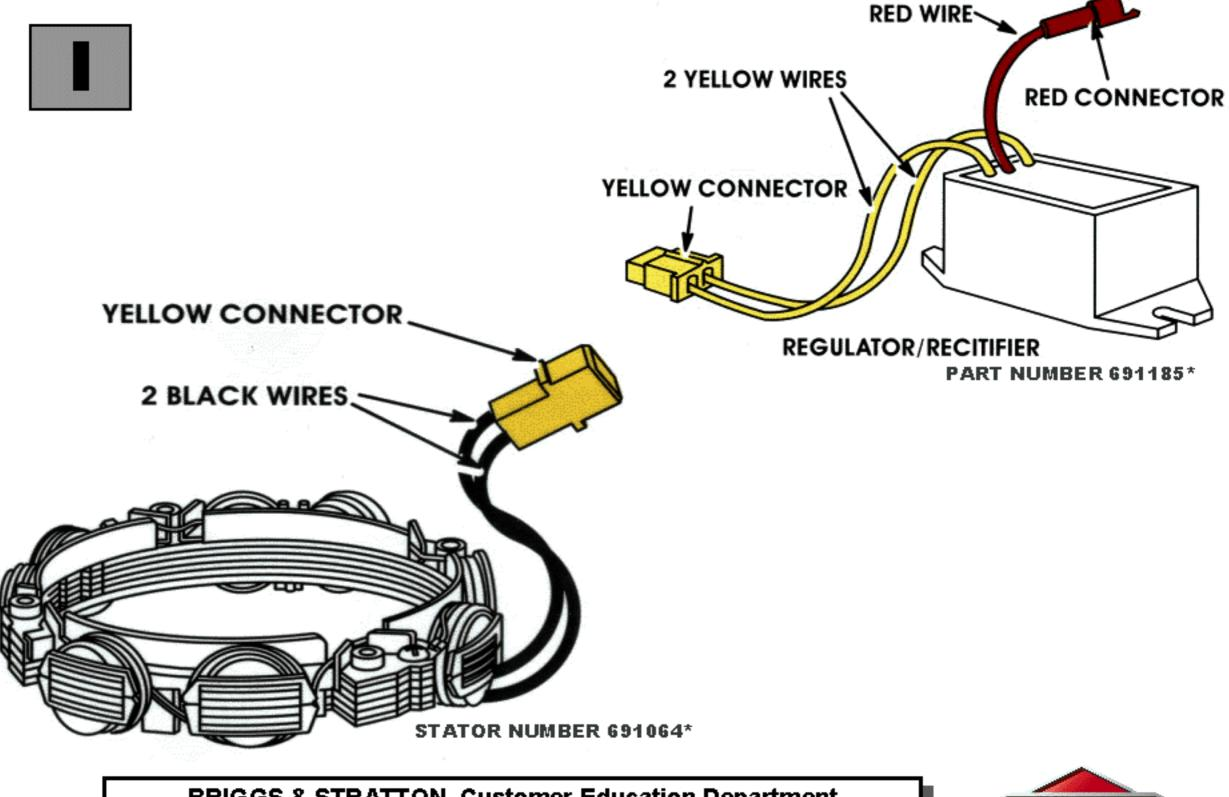
@ 3600 RPMs-16A Alternator 30 Volts AC(Min) at Stator; 16A, DC Regulated-red wire
