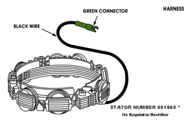
Tri-Circuit Alternator 28 Volts AC(Min) at 3600 RPM
