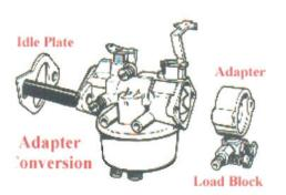
Air cooled engines run very efficiently on propane as their fuel source. When properly installed, it is clean burning and safe fuel to use. Keep in mind that you need to figure about 5% less power output when using propane than gasoline as a fuel. Over the last thirty plus years, I have often been involved in propane fueled engines on generators and various other equipment. I'll try and pass along some of the knowledge I have gained in this article.
