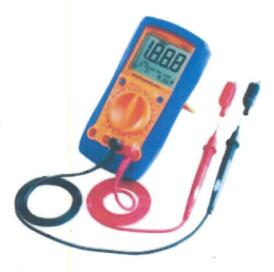
Set the meter to DC volts. Connect the voltmeter red lead to the post on the starter and the black lead to ground. Crank the engine and if it is below 9.5 volts,
