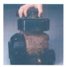
At this point you have decided the engine is smoking and needs a rebuild. I like to start by removing all the shrouding and use either compressed air or a pressure washer to clean the engine thoroughly before opening it up. You may want to take it to a car wash. This gives you a clean unit to work on. Leave the air filter on for this and duct tape the exhaust outlet and fuel cap vent. If you pressure wash the unit, blow dry with compressed air.
