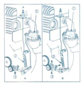
control the engine rpm's by varying the spring tension. All in all, it's a pretty simple device and for the most part very dependable.
