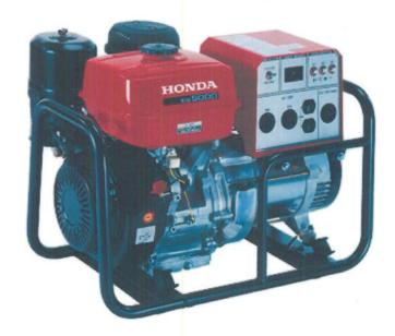
120 volts and put one on each circuit. The other thing you need to consider is many of the generators today are rated for maximum and continuous output. You want to run the load test at the continuous output rating. A 5000 watt unit might be rated 4500 watt or even 4000 watt continuous. You must get all this figured out before you run the load test.
